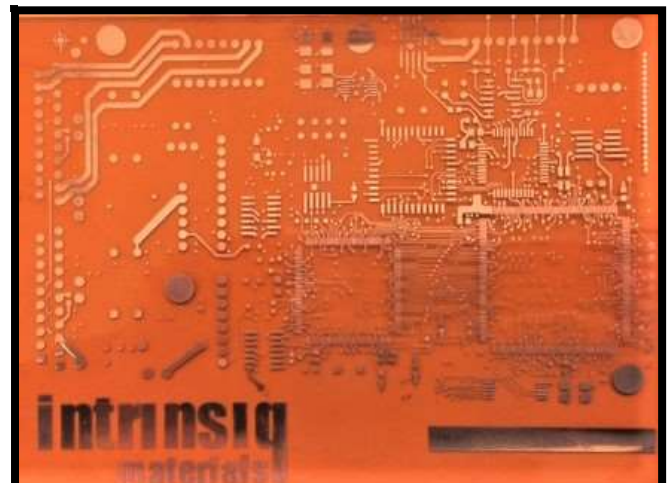
An image of CF-001 after copper film seed layer applied, photonic sintering, electroplating and etching
